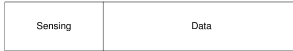
Figure 3.2: Time slot structure, showing the sensing period used by the relays to detect primary presence.
