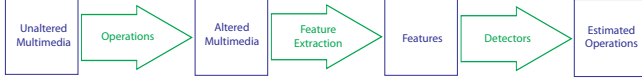
Fig. 1. Traditional process that a multimedia signal may go through when considering forensics.
