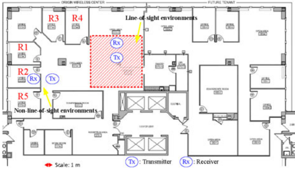
Fig. 9. Floor plan and the layout of the experiments in the LOS and NLOS testing environments. (Blue circles of Tx and Rx indicating the locations of the transmitter and the receiver, respectively).
