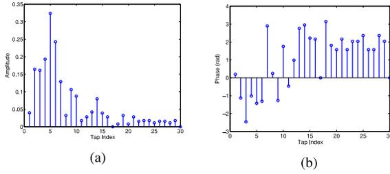
Fig. 4. Example of indoor CSI. (a) Amplitude of CSI. (b) Phase of CSI.
