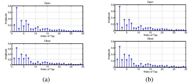
Fig. 8. Multipath profiles of door D1 under LOC B. (a) Multipath profiles (amplitude part) when TX on location 1 (NLOS). (b) Multipath profiles (amplitude part) when TX on location 5 (LOS).
